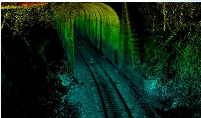
directly from the scan image. All other items can then be referenced in the scan relative to the track centreline. Any point can be assigned a chainage and horizontal and vertical offset along the track with respect to the plane passing through the two rail heads.
